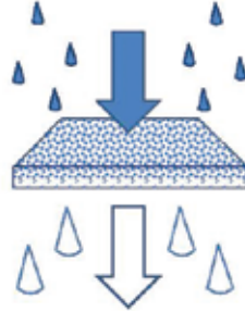
Fiberglass media is very efficient at removing solid contaminants and coalescing liquids out of natural gas.
